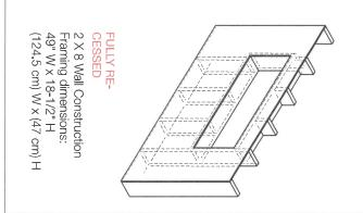
Must mount to a minimum of three (3) wall studs
