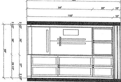
All dimensions given are subject to on-site verification and may be adjusted to suit job conditions. QTK reserves the right to modify the drawings or cabinet sizes as we deem fit. Customer acknowledges this drawing is to be used as a guide and should not order stone tops based solely on these dimensions.
