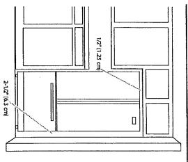
To ensure proper ventilation for your refrigerator, allow for a 1/2" (1.25 cm) space at the top and behind the refrigerator. If your refrigerator has an ice maker, allow extra space at the back for the water line connections. When installing your refrigerator next to a fixed wall, leave 2-1/2" (6.3 cm) minimum space between the refrigerator and wall to allow the door to swing open.
