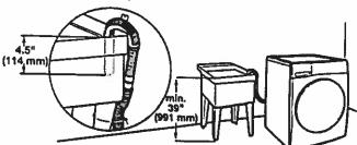
Minimum capacity: 20 gai. (76 L). Top of laundry tub must be at least 39" (991 mm) from the floor; install no higher than 96" (2.44 m) from bottom of washer.
