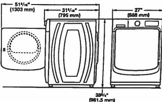
All dimensions show minimum spacing allowed. For each arrangement, consider allowing more space for ease of installation and servicing, and spacing for companion appliances and clearances for walls, doors, and floor moldings.
