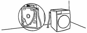
Floor drain system requires a Siphon Break Kit, two Connector Kits, and an Extension Drain Hose that may be purchased separately. Please contact your retailer for ordering information, or see the "Assistance or Service" page on the back of your Use and Care Guide, Minimum siphon break height: 28° (710 mm) from bottom of washer. (Additional hoses may be needed.)
