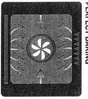
The European convection system ensures even roasting and baking on multiple levels with no flavor crossover.
