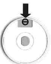
Adjustment screw next to the valve shaft Fig. 3
