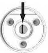
Center adjustment screw Fig. 2
