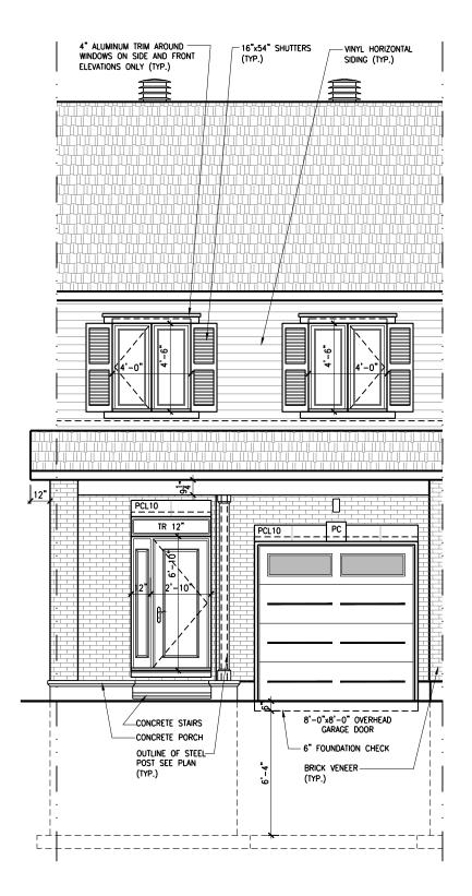
FRONT ELEVATION - MID UNIT ( A.1b SCALE: 3/16" = 1'-0"
