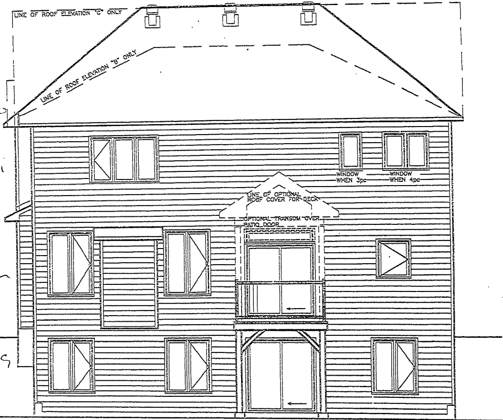
REAR ELEVATION c/w WALK OUT BASEMENT
