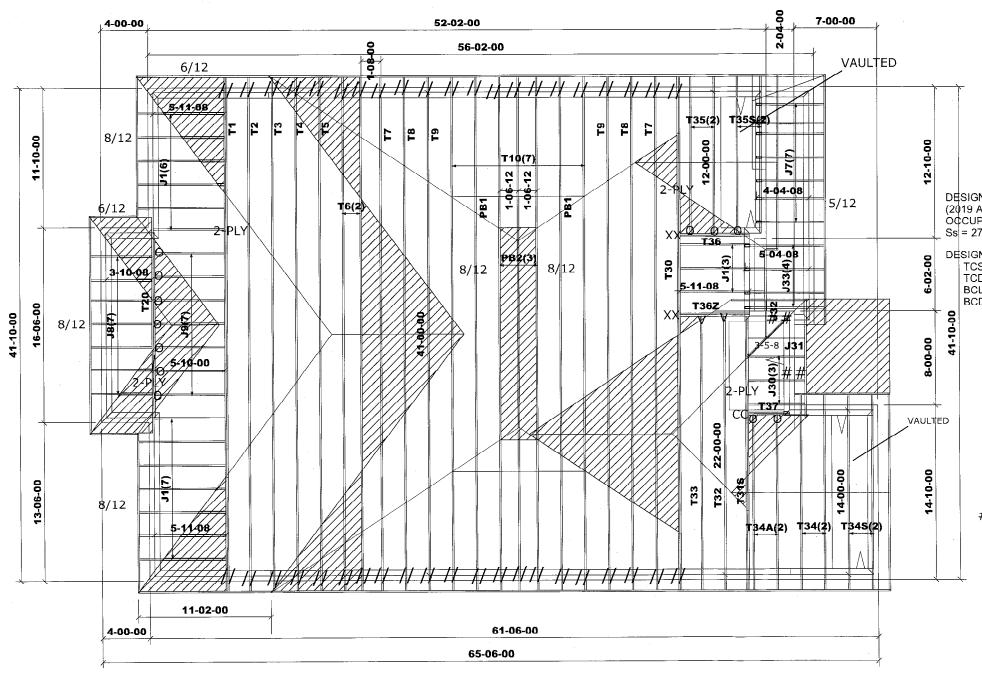
All conventional framing to conform with Part 9 of O.B.C. 2012 (2019 amendment). Roof rafters that cross over or meet trusses to be min. 2x4 SPF #2 @ 24" o/c with a vertical post to the truss at each cross point. Vertical posts longer than 6' to have lateral bracing so that the distance between the post end points and lateral bracing does not exceed 6'.
