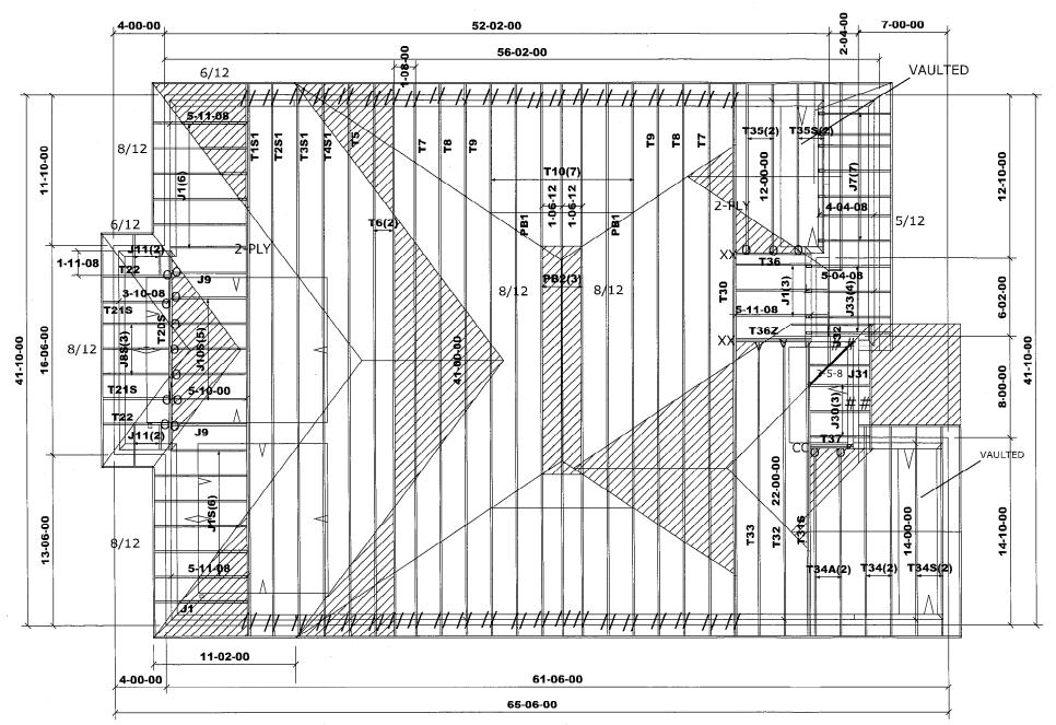
All conventional framing to conform with Part 9 of O.B.C. 2012 (2019 amendment). Roof rafters that cross over or meet trusses to be min. 2x4 SPF #2 @ 24" o/c with a vertical post to the truss at each cross point. Vertical posts longer than 6' to have lateral bracing so that the distance between the post end points and lateral bracing does not exceed 6'.
