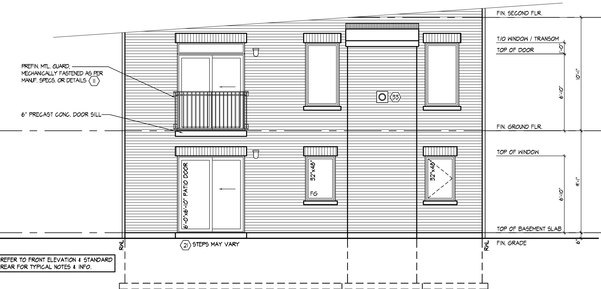
PART. REAR ELEVATION - W.O.B. CONDITION
