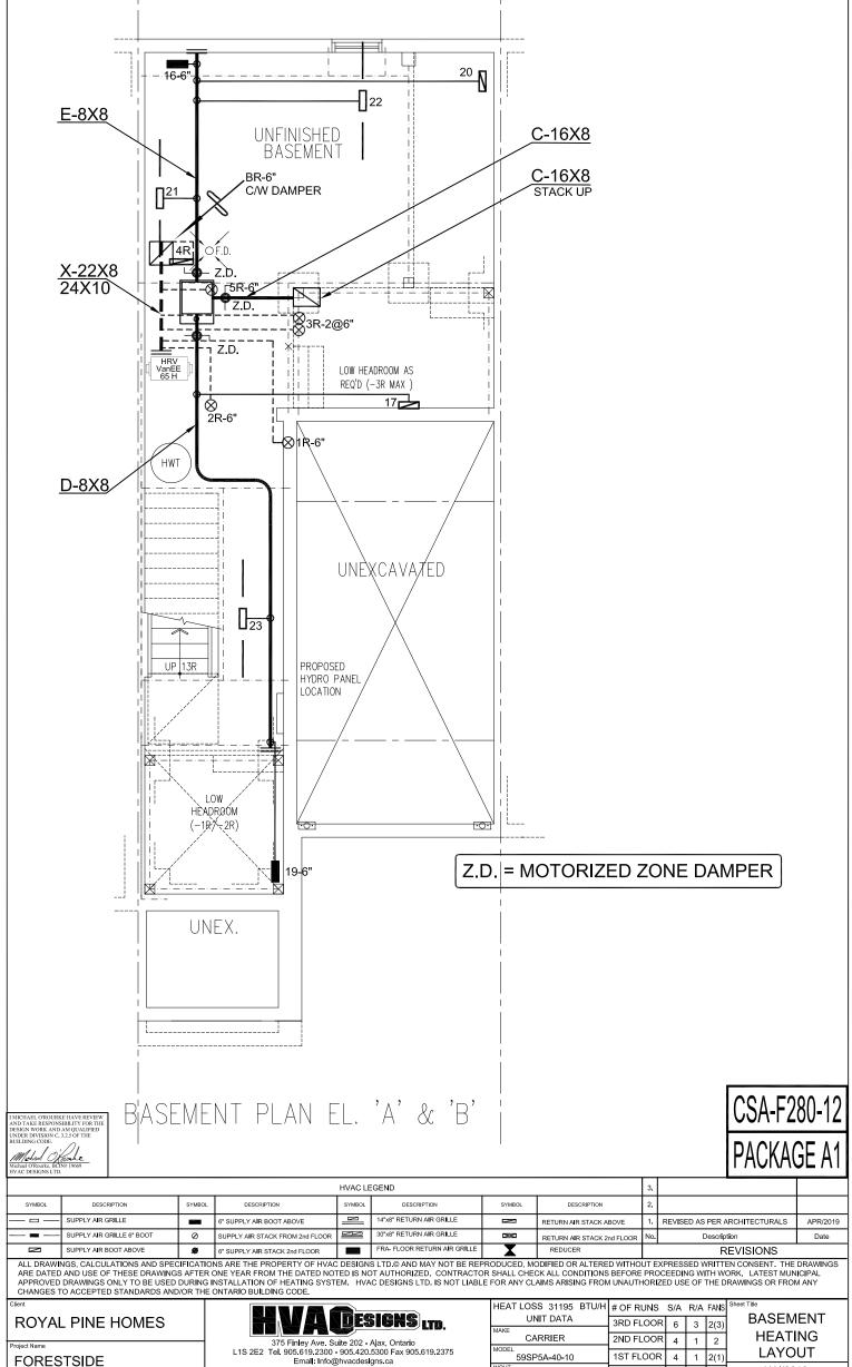
JAN/2018 BASEMENT 3 1 0 BRAMPTON, ONTARIO ALL S/A DIFFUSERS 4 "x10" UNLESS NOTED OTHERWISE ON LAYOUT. ALL S/A RUNS 5 UNLESS NOTED OTHERWISE ON LAYOUT. UNDERCUT DOORS 1" min. FOR R/A Installation to comply with the latest Ontario Building Code. All supply branch outlets shall be equipped with a manual balancing damper.
