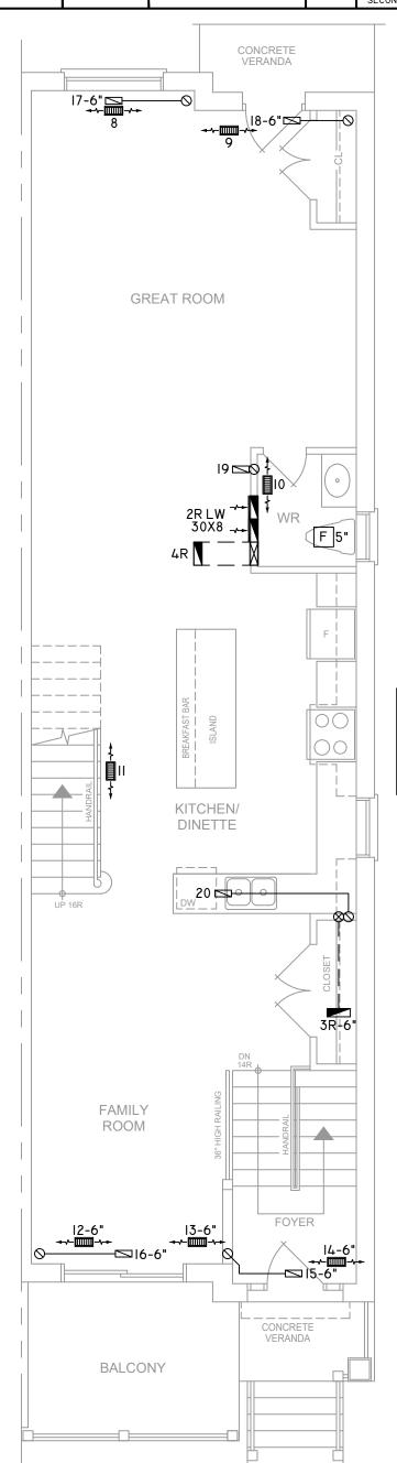
KITCHEN EXHAUST 100 CFM MIN. 6" ALL OTHER FANS SHALL BE A MIN. OF 50 CFM OR OTHERWISE NOTED AS PER 9.32.3.5
