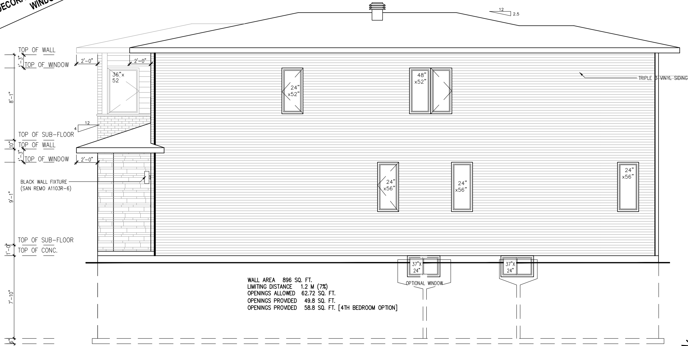
RIGHT SIDE ELEVATION ELEVATION M
