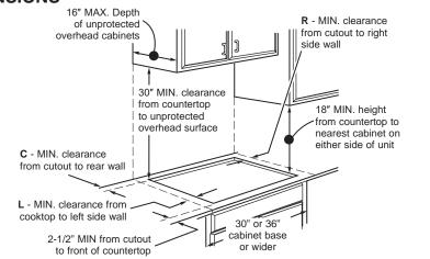
ALL HORIZONTAL **CLEARANCES MUST** BE MAINTAINED FOR A **MINIMUM OF 18" ABOVE** THE COOKING SURFACE
