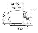
$\label{eq:local_commonded} \begin{tabular}{ll} $(\mbox{$4$}\mbox{$0$}): Recommended faucet area of 15" (L) x 4" (W). Depth recommended for straight pipes 8". All dimensions are approximate. Structure measurements must be verified against the unit to ensure proper fit. \\ \end{tabular}$
