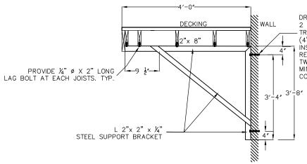
DRILL INTO EXISTING FOUNDATION WALL 2 -1/2" Ø RED HEAD STAINLESS STEEL TRUBOLT WEDGE ANCHOR (4" MIN. EMBEDMENT) INSTALL AS PER MANUFACTURERS RECOMMENDATIONS. TWO BOLTS PER BRACKET LEG. MIN. EDGE DISTANCE FROM TOP OF CONCRETE WALL=4"
