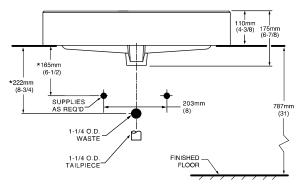
NOTES: \*DIMENSIONS SHOWN FOR LOCATION OF SUPPLIES AND "P" TRAP ARE SUGGESTED. FAUCETS NOT INCLUDED WITH FIXTURE AND MUST BE ORDERED SEPARATELY. FOR COUNTERTOP CUTOUT AND INSTALLATION INSTRUCTIONS USE TEMPLATE SUPPLIED WITH SINK,
