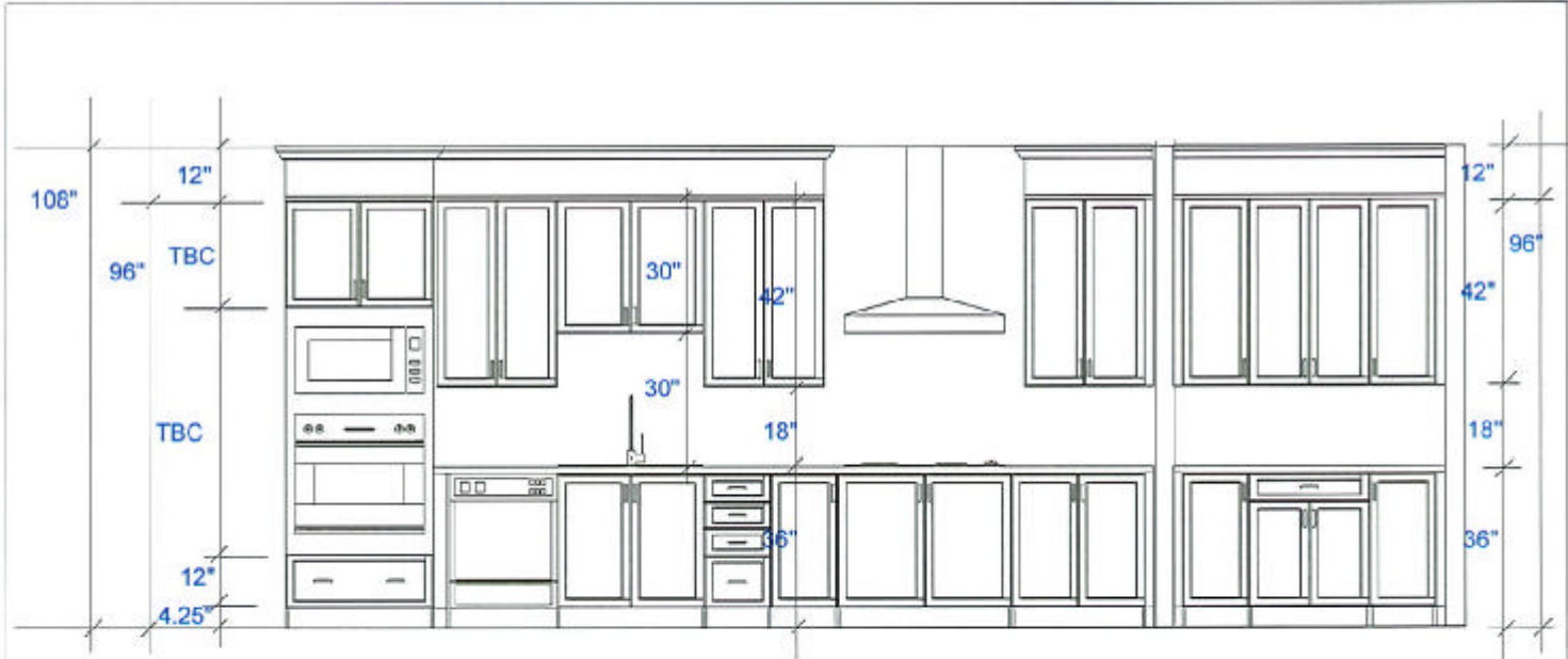
OVEN / SINK / COOKTOP WALL ELEVATION BUTLER'S PANTRY
