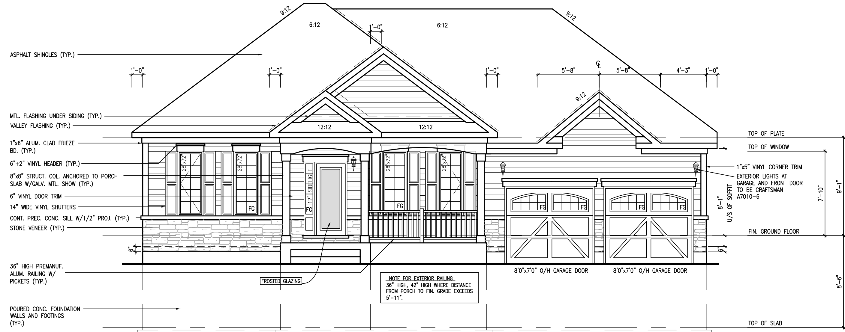
FRONT ELEVATION 'A' (SIDING W/ STONE BASE)
