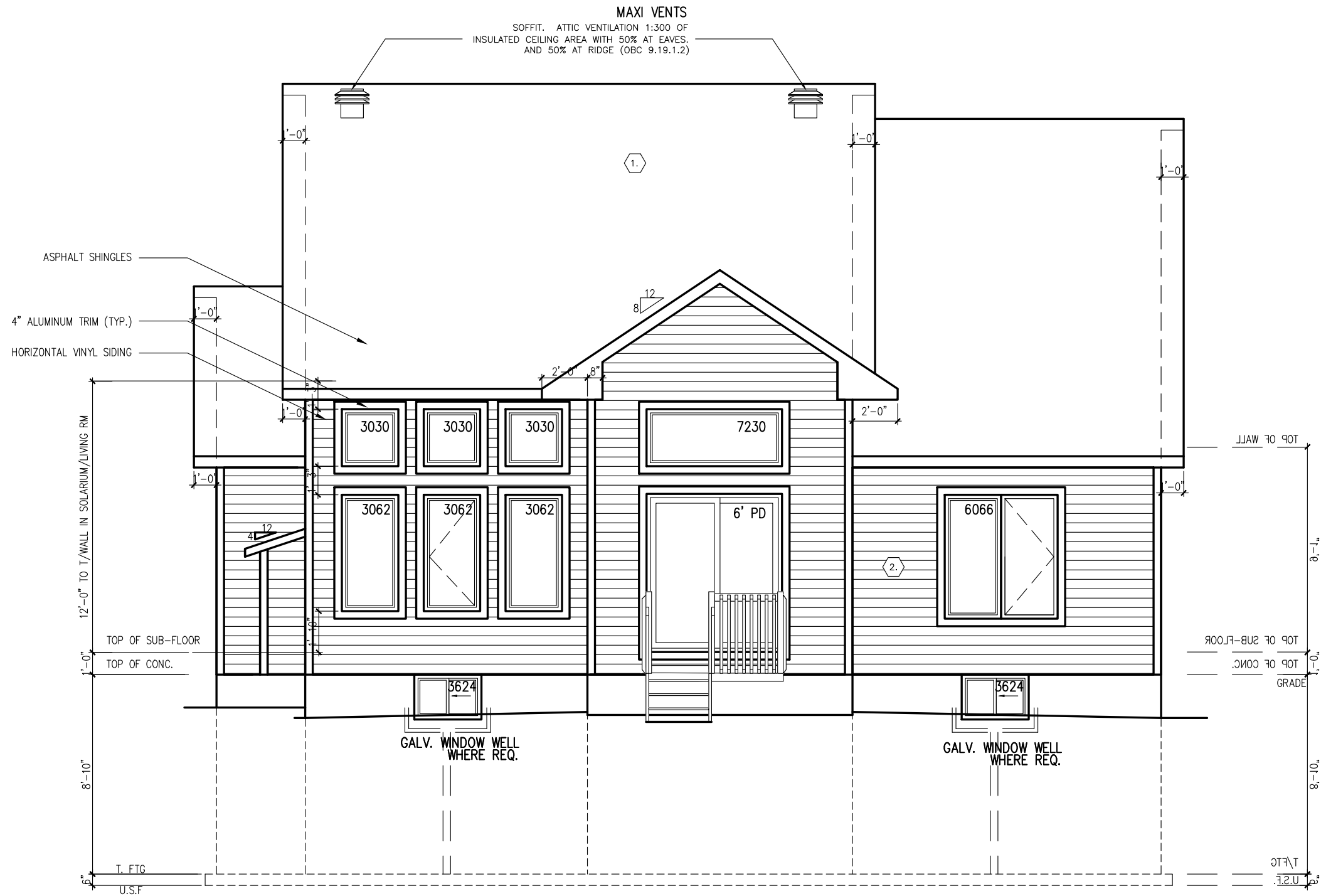
ELEVATION C SUN ROOM REAR ELEVATION
