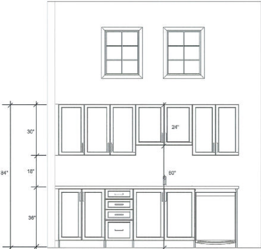
SINK WALL ELEVATION DCR - SPRINGFIELD STANDARD KITCHEN
