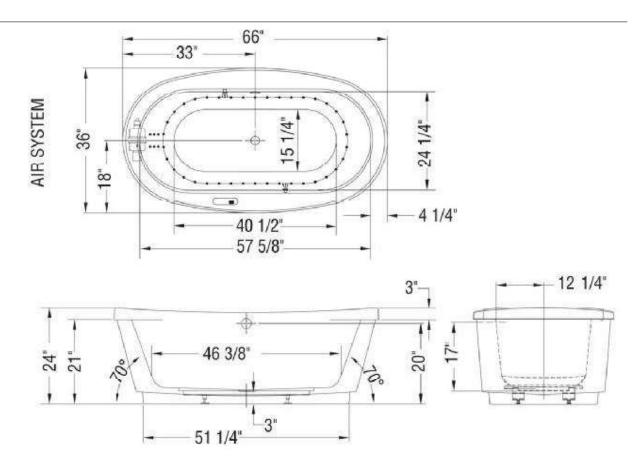
( • ): Indicates airjets positioning ( 聖 ): Indicates chromatherapy light positioning All dimensions are approximate. Structure measurements must be verified against the unit to ensure proper fit.
