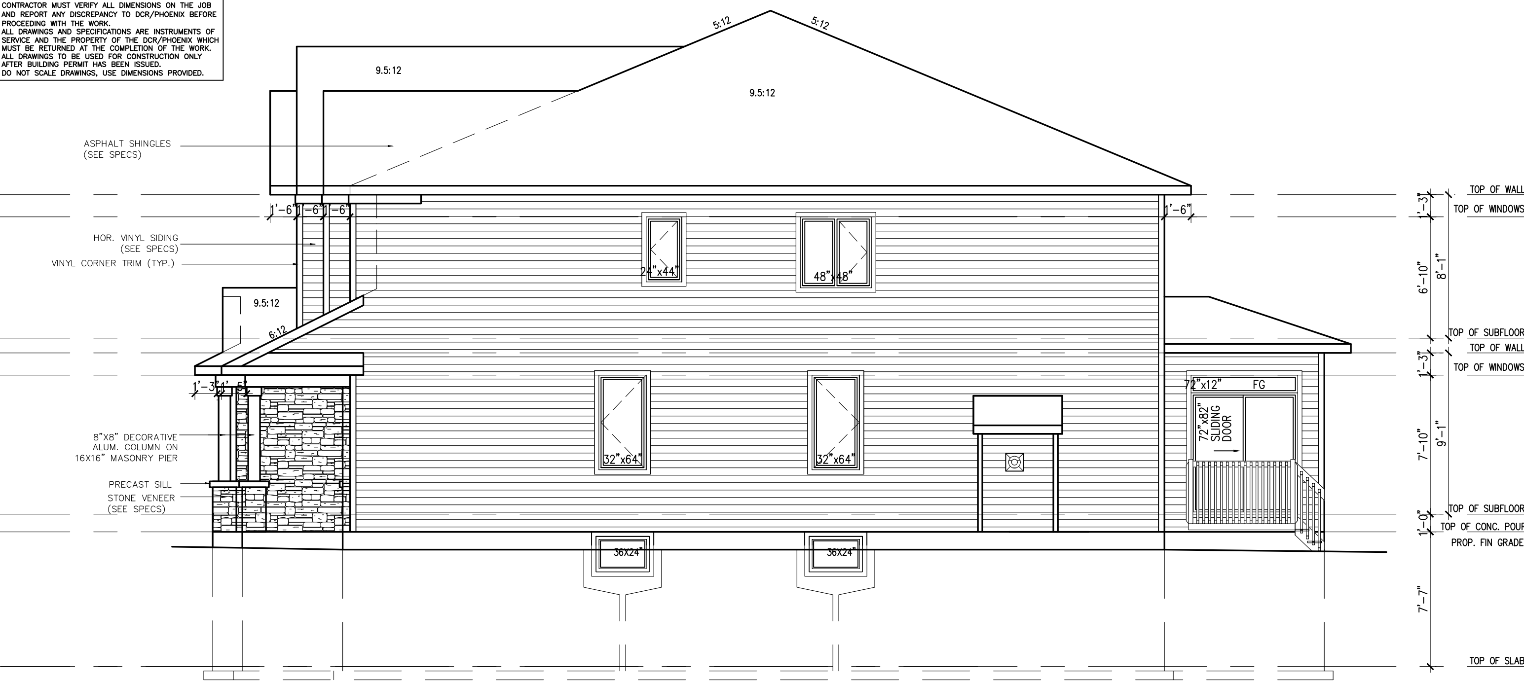
RIGHT SIDE ELEVATION-A (4 BEDROOM)
