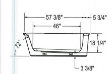
(a): Recommended faucet area 2 sections of 12" (L)  $\times$  3 1/2" (W). All dimensions are approximate. Structure measurements must be verified against the unit to ensure proper fit.
