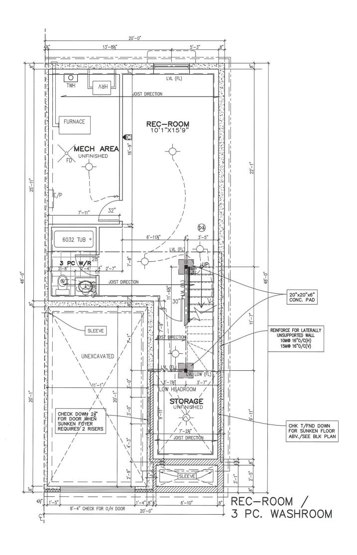
\*\*NOTE\*\* ALL WINDOW, DOOR & O/H GARAGE DOOR LINTELS TO BE 2-2X10 W/ P2 POSTS ON EACH SIDE U.N.O.
