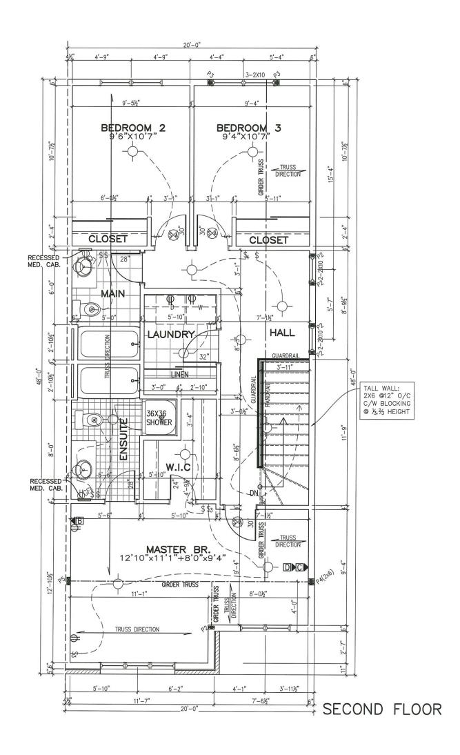
\*\*NOTE\*\* ALL WINDOW, DOOR & O/H GARAGE DOOR LINTELS TO BE 2-2X10 W/ P2 POSTS ON EACH SIDE U.N.O.
