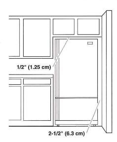
To ensure proper ventilation for your refrigerator, allow for 1/2" (1.25 cm) space at the top and behind the refrigerator. If your refrigerator has an ice maker, allow extra space at the back for the water connections. When installing your refrigerator next to a fixed wall, leave 2 1/2" (6.3 cm) minimum on each side (some models require more) to allow for the door to swing open.
