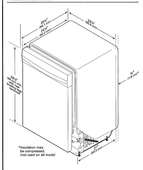
**NOTE:** Shaded area of cabinet walls show where utility connections may be installed.
