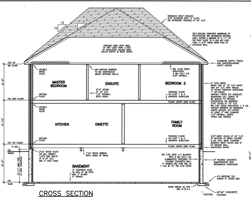
MINIMUM FOOTING WIDTH OR AREA SHALL CONFORM TO TABLE 9.15.3.4.
