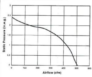
HVI-2100 CERTIFIED RATINGS comply with new testing technologies and procedures prescribed by the Home Vantilating Institute, for off-the-shell products, as they are available to consumers. Product performance is rated at 0.1 in. static pressure, based on tests conducted in AMCA's state-of-the-art test laboratory. Sones are a measure of humanly-perceived loudness, based on laboratory measurements.
