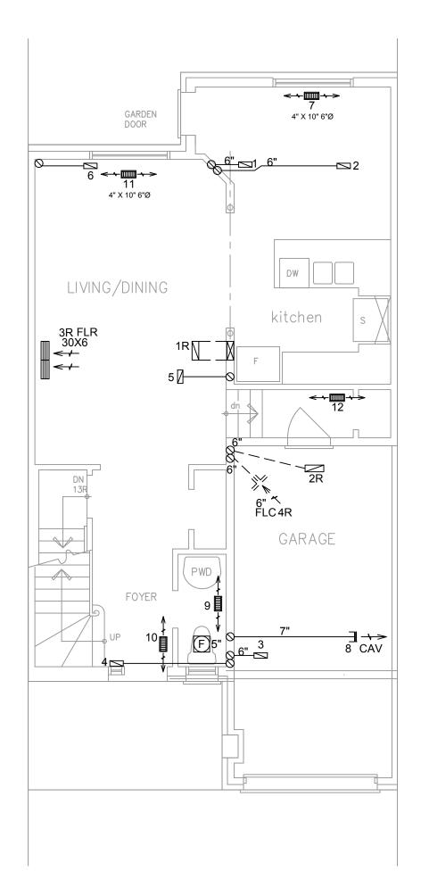
INSULATE ALL DUCTS IN UNCONDITIONED SPACES MIN. R12
