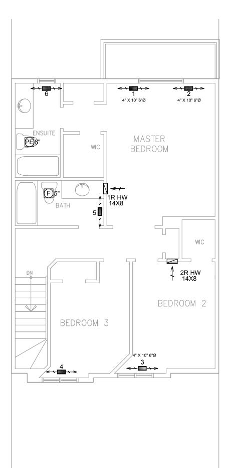
INSULATE ALL DUCTS IN UNCONDITIONED SPACES MIN. R12
