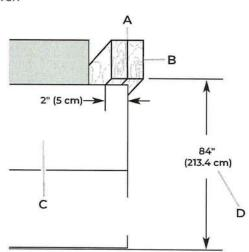
A. Two 2"  $\times$  4"  $\times$  32" (5 cm  $\times$  10 cm  $\times$  81 cm) boards B. Attach to studs with six #8  $\times$  3" (7.6 cm) screws.
