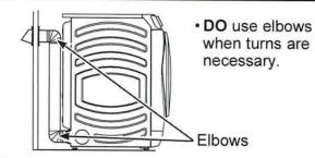
DO NOT bend or collapse ducting.
