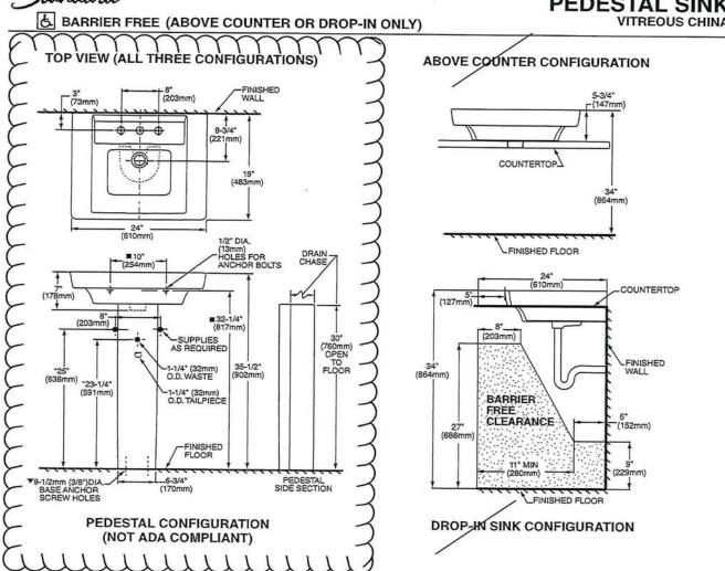
ABOVE COUNTER AND DROP-IN SINK CONFIGURATIONS MEET THE AMERICANS WITH DISABILITIES ACT GUIDELINES AND ANSI A117.1 ACCESSIBLE AND USABLE BUILDINGS AND FACILITIES - CHECK LOCAL CODES. Top of sink installed at 34" (864mm) height from finished floor. Sink installed 5" (127mm) minimum from front edge of countertop. Provide 27" (686mm) knee clearance area.
