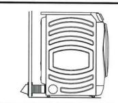
DO cut duct as short as possible and install straight into wall.
