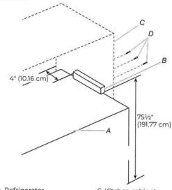
A. Refrigerator B. Secondary anti-tip board
