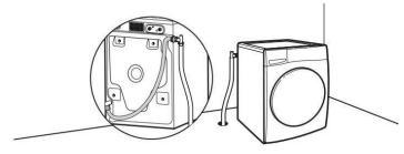
Floor drain system requires a Siphon Break Kit, 2 Connector Kits, and an Extension Drain Hose that may be purchased separately; refer to the Quick Start Guide for online ordering information. Minimum siphon break height: 28" (710 mm) from bottom of washer. (Additional hoses may be needed.)
