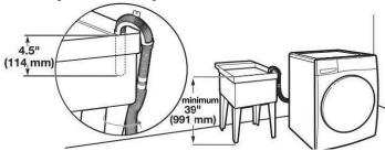
Minimum capacity: 20 gallons (76 L). Top of laundry tub must be at least 39" (991 mm) from the floor; install no higher than 96" (2.4 m) from bottom of washer.
