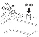
that the drain hose either be looped up and securely fastened to the underside of the counter or be connected to an air gap.
