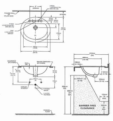
\*\* DIMENSIONS SHOWN FOR LOCATION OF SUPPLIES AND "P" TRAP ARE SUGGESTED. FOR COUNTERTOP CUTOUT AND INSTALLATION INSTRUCTIONS USE TEMPLATE FOR COUNTERTOP CUTOUT AND INSTALLATION INSTAUCTIONS USE TENTE STEE SUPPLIED WITH SINK.
