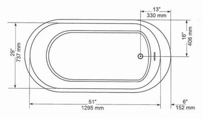
GENERAL SPECIFICATIONS Average Weight 90 lb 41 kg Bathing Well at bottom 1092 x 508 mm 43"x 20" Capacity Drain to Overflow 195 litres Water Depth Drain to Overflow 16" 406 mm Drain Opening (dia.) 51 mm
