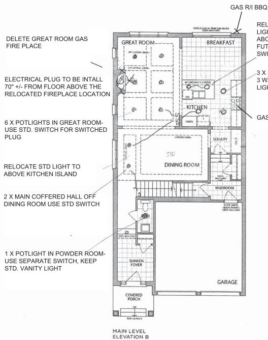
RELOCATE KITCHEN LIGHT AND HALLWAY LIGHT TO BE CAPPED CEILING LIGHT ABOVE THE BREAKFAST BAR FOR FUTURE PENDANT LIGHTS ON SEPARATE SWITCH
