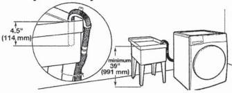
Minimum capacity: 20 gallons (76 L). Top of laundry tub must be at least 39" (991 mm) from the floor; install no higher than 96" (2.4 m) from bottom of washer.
