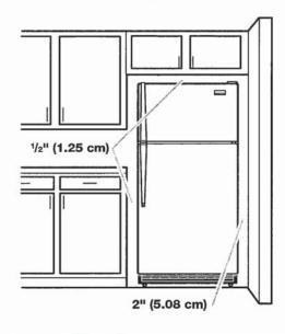
To ensure proper ventilation for your refrigerator, allow for a ½" (1.25 cm) space on each and between overhead cabinets and refrigerator top. Allow at least 1" (2.5 cm) between back of cabinet and the wall. If your refrigerator has an ice maker, make sure you leave some extra space at the back for the water line connections.
