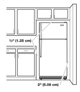
To ensure proper ventilation for your refrigerator, allow for a  $\frac{1}{2}$ " (1.25 cm) space on each and between overhead cabinets and refrigerator top. Allow at least 1" (2.5 cm) between back of cabinet and the wall. If your refrigerator has an ice maker, make sure you leave some extra space at the back for the water line connections.
