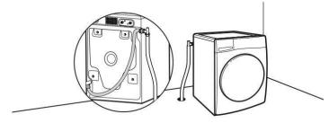
Floor drain system requires a Siphon Break Kit, 2 Connector Kits, and an Extension Drain Hose that may be purchased separately; refer to the Quick Start Guide for online ordering information. Minimum siphon break height: 28" (710 mm) from bottom of washer. (Additional hoses may be needed.)
