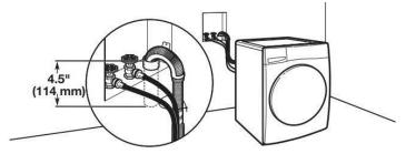
See requirements in "Floor standpipe drain system."
