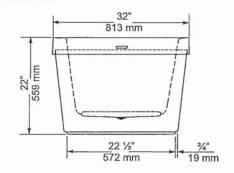
GENERAL SPECIFICATIONS 90 lb Average Weight 41 kg Bathing Well at bottom 43"x 20" 1092 x 508 mm Capacity Drain to Overflow 195 litres Water Depth Drain to Overflow 16" 406 mm Drain Opening (dia.) 51 mm 2 1/4"x 1/2" Overflow Opening 57 x 13 mm Drain to Floor Clearance 3 1/4" 83 mm
