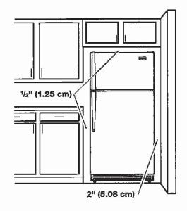
To ensure proper ventilation for your refrigerator, allow for a %" (1.25 cm) space on each and between overhead cabinets and refrigerator top. Allow at least 1" (2.5 cm) between back of cabinet and the wall. If your refrigerator has an ice maker, make sure you leave some extra space at the back for the water line connections.
