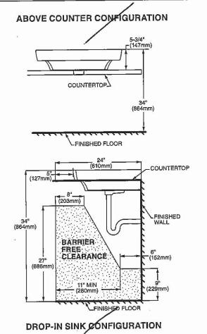
ABOVE COUNTER AND DROP-IN SINK CONFIGURATIONS MEET THE AMERICANS WITH DISABILITIES ACT GUIDELINES AND ANSI A117.1 ACCESSIBLE AND USABLE BUILDINGS AND FACILITIES - CHECK LOCAL CODES. Top of sink installed at 34" (864mm) height from finished floor.
