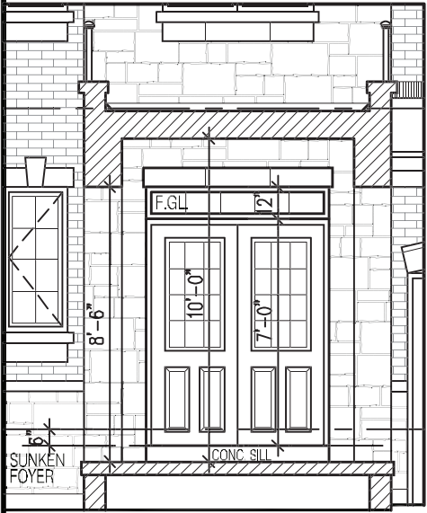
PORTICO INTERIOR ELEVATION 2
