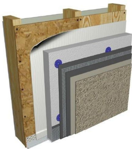
Figure 7. InsulROCK EIFS over modified bituminous membrane on OSB and plywood
