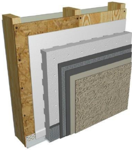
Figure 10. Puccs EIFS with moisture barrier over OSB and plywood
