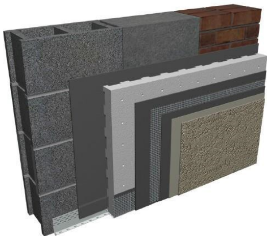
Figure 6. InsulROCK EIFS over modified bituminous membrane on masonry, concrete, and brick
