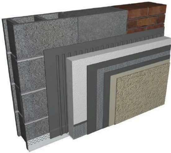
Figure 4. InsulROCK EIFS with moisture barrier over masonry, concrete, and brick
