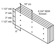
FOR 4 PLY BEAMS\*, ATTACH PLIES TOGETHER USING 6-3/4" SDW SCREWS (HEAD ON LOADED SIDE) IN 3 ROWS @ 16" C/C.
