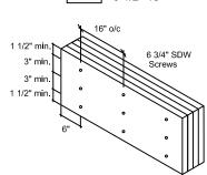
FOR 4 PLY BEAMS\*, ATTACH PLIES TOGETHER USING 6-3/4" SDW SCREWS (HEAD ON LOADED SIDE) IN 3 ROWS @ 16" C/C.
