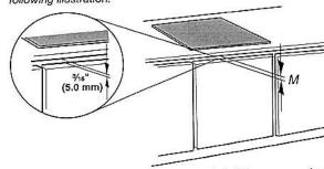
NOTES: After you make the countertop cutout, some installations may require notching down the base cabinet side walls to clear the cooktop base. To avoid this modification, use a base cabinet with sidewalls wider than the cutout.
