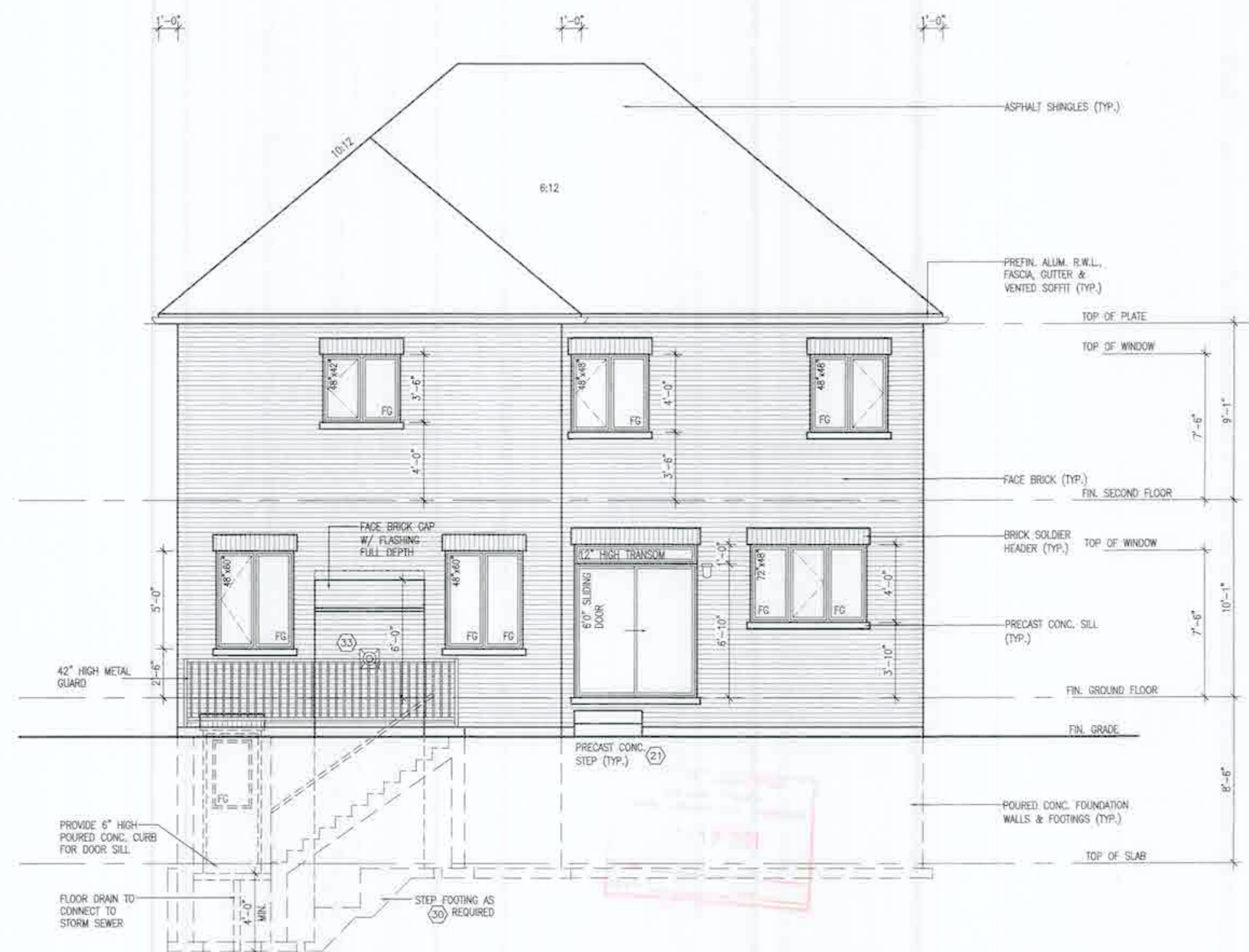
REAR ELEVATION '1' WALK-UP BASEMENT CONDITION
