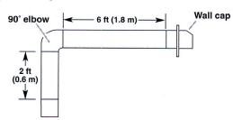
The following example falls within the maximum recommended vent length of  $35\ \text{ft}\ (10.7\ \text{m}).$
