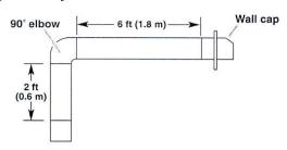
The following example falls within the maximum recommended vent length of 35 ft (10.7 m).
